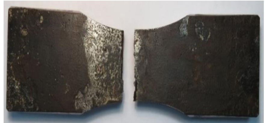
View of destroyed specimens after fatigue tests on the UMM-01 installation
