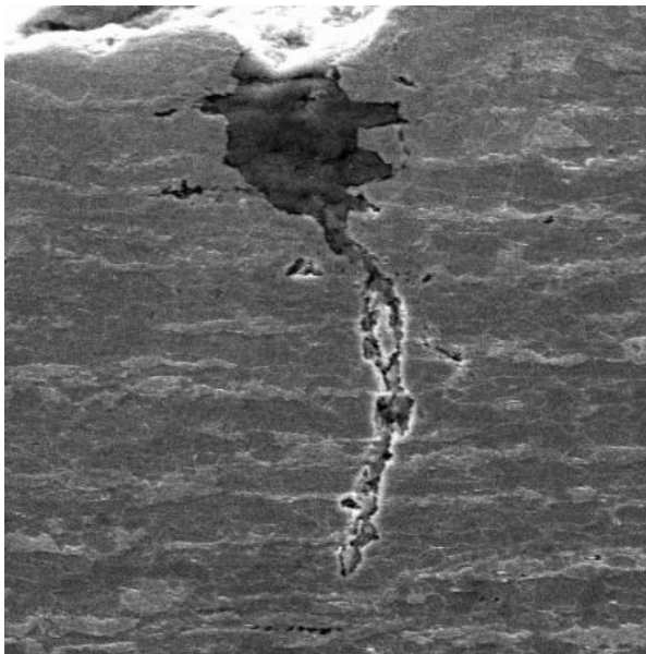
Electronic image of stress corrosion crack
