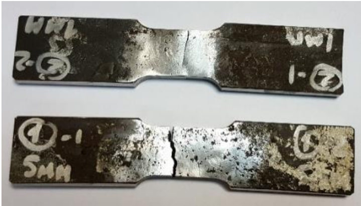
View of destroyed specimens after fatigue tests on the UMP-01 installation
