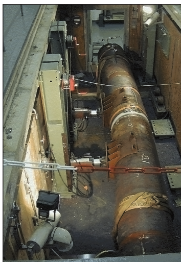
Fig. 8. Rupture pit to carry out sustained pressure tests
